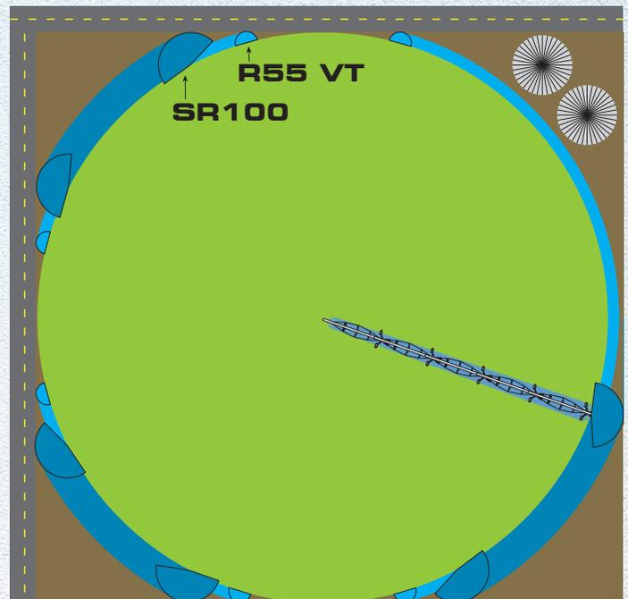
A secondary end gun can pick up extra acres by irrigating where the SR100 can't – as the pivot enters/exits the corner, and around obstacles such as roads and buildings.
