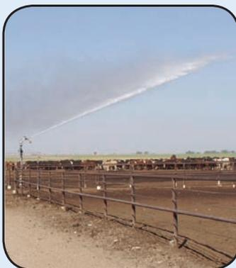
Nelson Big Gun® sprinklers are ideal for feedlot dust suppression and cooling applications. With a full range of models available (see *The Original Big Gun®* brochure), flow rates of 30-1200 GPM (6.8-275 m<sup>3</sup>/hr) can be achieved with maximum uniformity to match a variety of needs. Uniformity of coverage is important to prevent standing water. Overwatering causes odor problems that can be more troublesome than dust.
